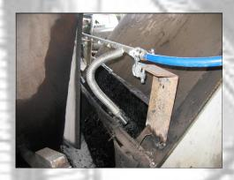
Easy to install and maintain, BG's spray bars clamp to the outside of the system and are easily removed for access to the slats. Operation is a snap, with control valves running spray bars and guns efficiently and safely.
